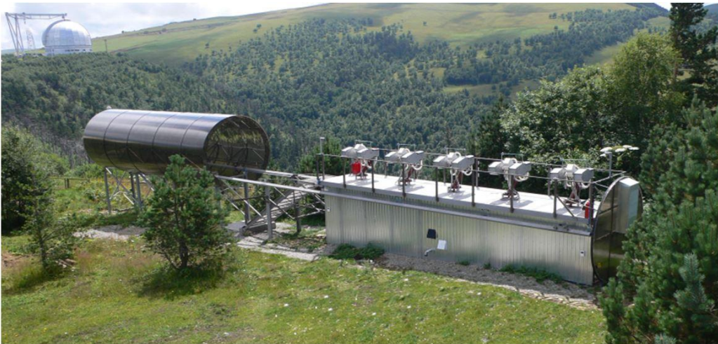
Fig2. Photo of all 9 channels of MMT installed on 5 mounts in the single cylindrical dome, which is open at that moment. The dome of the Russian 6-m telescope is seen in the background.
